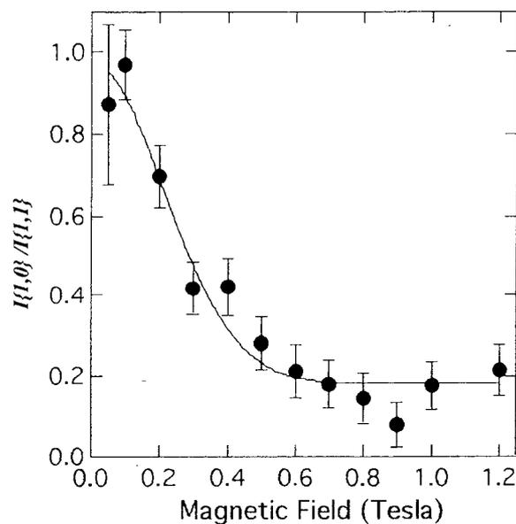
FIG.1: Ratio of the hexagonal  $\{1,0\}$  to quadratic  $\{1,1\}$  intensity spots of SANS in a single crystal of  $\text{La}_{1.83}\text{Sr}_{0.17}\text{CuO}_{4+\delta}$  as a function of a magnetic field along the c-axis. The leveling off near 0.4 Tesla is marked. Adapted from Fig.4 of Ref. 8 and Fig. 3b of Ref. 5
