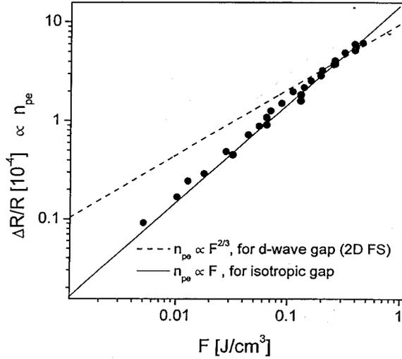
Fig.2: Ratio of the reflectivity change  $\Delta R/R$  in optical pulsed experiments in YBCO as a function of the fluence  $F$  of the first pulse, the second second being the probing pulse. The data are from two different laboratories [25,26] plotted by J. Demsar. Included is also the expected fluence dependence  $F^{2/3}$  for d- as well as  $F$  for s-symmetry.
