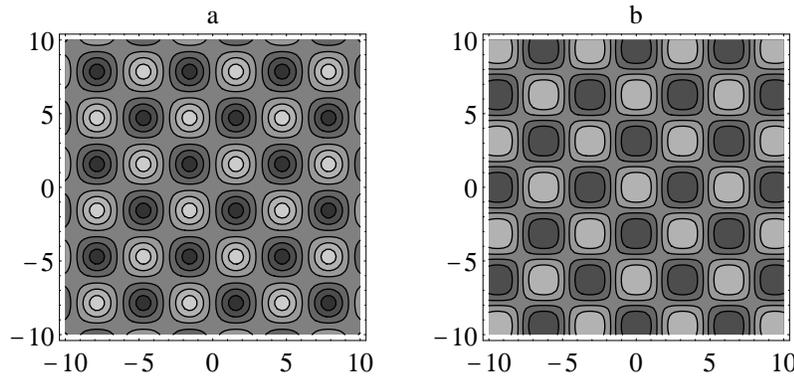
**Figure 3.** Contour plots of the Bloch states at the corner  $k_x = 1, k_y = 1$  of the BZ for the lower (a) and upper (b) band of figure 1. The wavefunction in (a) leads to soliton formation through modulational instability while the one in (b) is modulationally stable.
