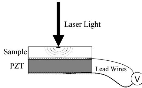
Figure 1: Schematic configuration of a  $\text{CsPbCl}_3$  and a PZT. The sample was photoexcited on one cleaved plane and PA signals were detected on the other by the PZT attached with conductive organic paste. Dotted lines in the sample stand for the PA waves schematically. The piezoelectric voltage was measured along the thickness direction. This figure is drawn for the PZT of  $5 \times 5 \times 1 \text{ mm}^3$ . More details are described in Sec. 2.
