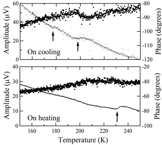
Figure 4: Amplitude (closed circle) and phase (dot) of PA signal vs temperature. The incident light was 10-Hz and 3.49-eV pulsed laser light and the incident direction was parallel to  $c$  axis. The resonant frequency of PZT was 1.97 MHz. The increasing and decreasing rates of temperatures were 1.2 K/min. Arrows indicate the lower edge of phase change and are indicative of phase transitions; the discussion on phase transitions is given in Sec. 4.
