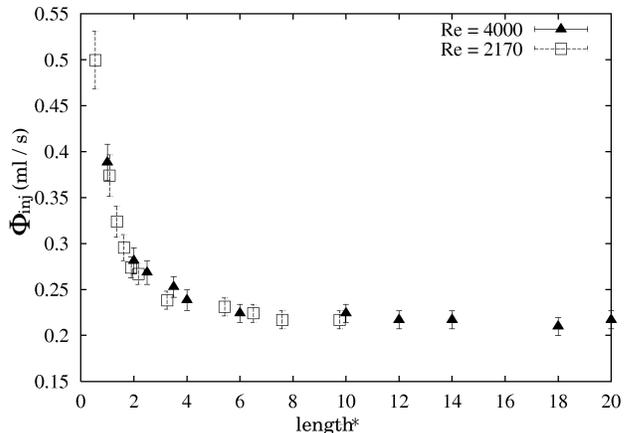
FIG. 3: Stability curves measured for  $Re = 2170$  and  $Re = 4000$ . Each data point was obtained from forty runs of the experiment and the error bars correspond to the widths of the determined probability distributions [8]. The abscissa is the ‘ $length^*$ ’ of the initially disturbed flow in pipe diameters.
