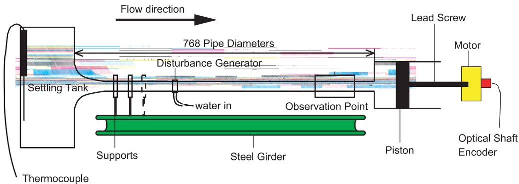
FIG. 1: Schematic of the ‘long pipe’ experimental system.
