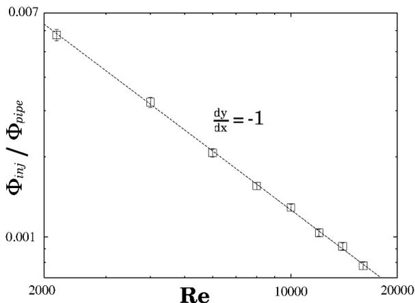
FIG. 5: A log-log plot of the stability curve obtained using the long pipe. The range of  $Re$  covered is 2000 to 18,000 and the amplitude of the perturbation has been non-dimensionalized by the respective mass flux in the pipe. The least squares fitted line has a slope of -1 as indicated.
