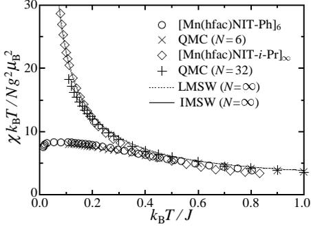
FIG. 3. Magnetic-susceptibility measurements on [Mn(hfac)NIT-Ph]<sub>6</sub> at  $H = 0.5$  T [15] and on [Mn(hfac)NIT-*i*-Pr]<sub>∞</sub> at  $H = 0$  [16] compared with quantum Monte Carlo calculations (QMC). They are in good agreement assuming  $J/k_B \simeq 370$  K for [Mn(hfac)NIT-Ph]<sub>6</sub> and  $J/k_B \simeq 360$  K for [Mn(hfac)NIT-*i*-Pr]<sub>∞</sub>. Linear (LMSW) and interacting (IMSW) modified spin-wave calculations at  $N = \infty$  are also shown.
