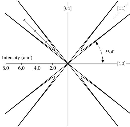
FIG. 9: Angular distribution of radiative power corresponding to the normalized frequency  $\Omega = 0.34$ . The directions of infinite radiative power (caustic) coincide with the directions of the folds of the wave contour (Fig. 8).
