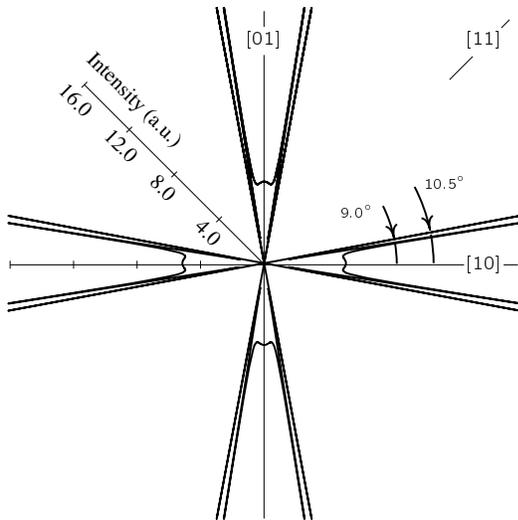
FIG. 13: Angular distribution of radiative power corresponding to the normalized frequency  $\Omega = 0.565$ . The directions of infinite radiative power (caustic) coincide with the directions of the folds of the wave contour.
