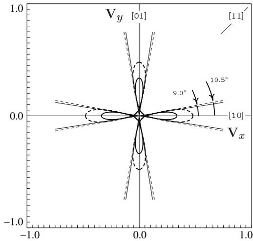
FIG. 12: Wave contours corresponding to the normalized frequency  $\Omega = 0.565$ . Solid (dashed) wave contour corresponds to solid (dashed) iso-frequency contour in figure 11. The group velocity is plotted in the units of the speed of light in vacuum. The directions corresponding to the folds of the wave contour are shown.
