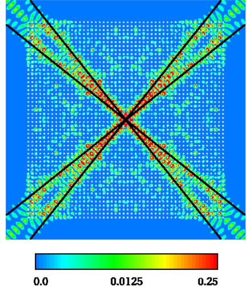
FIG. 10: FDTD calculation. Map of the modulus of the Poynting vector field for a  $50 \times 50$  rod photonic crystal excited by a point isotropic source with the normalized frequency  $\Omega = 0.34$ . The location of the crystal in the simulation is shown together with asymptotic directions of photon focusing caustics.
