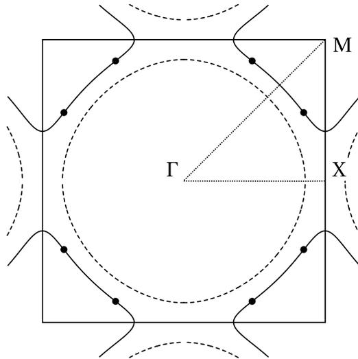
FIG. 5: Iso-frequency contours of the square lattice photonic crystal for the normalized frequencies  $\Omega = 0.31$  (dashed line) and  $\Omega = 0.34$  (solid line). Parabolic point are marked by the black dots. The first Brillouin zone of the lattice is plotted in order to show the spatial relation between zone boundary and iso-frequency contours.
