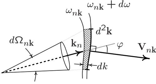
FIG. 1: Diagram showing the relations between  $\mathbf{k}$ -space and coordinate space quantities. Iso-frequency contours for frequencies  $\omega_{n\mathbf{k}}$  and  $\omega_{n\mathbf{k}} + d\omega$  are presented.
