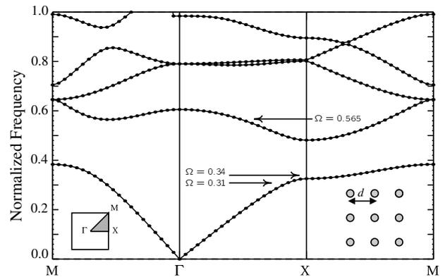
FIG. 4: Photonic band structure of TM modes for the square lattice photonic crystal with refractive index of the rods  $n = 2.9$ , the lattice constant  $d$  and radius of the rods  $0.15d$ . The frequency is normalized to  $\Omega = \omega d/2\pi c = d/\lambda$ .  $c$  is the speed of light in vacuum. Insets show the first Brillouin zone of the crystal with the irreducible zone shaded light gray (left) and a part of the lattice (right).
