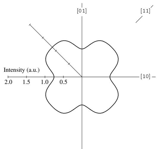
FIG. 7: Angular distribution of radiative power corresponding to the normalized frequency  $\Omega = 0.31$ . High symmetry directions of the square lattice are specified.
