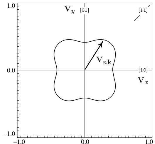
FIG. 6: Wave contour corresponding to the normalized frequency  $\Omega = 0.31$ . The group velocity is plotted in the units of the speed of light in vacuum. High symmetry directions of the square lattice are specified.
