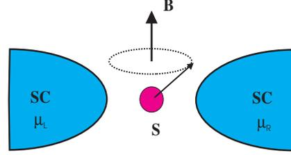
FIG. 1: Magnetic spin coupled to two superconducting leads. In the presence of a magnetic field  $\mathbf{B}$ , the spin precesses around the field direction. As we illustrate here, in a Josephson junction the standard precession is accompanied by a polar motion leading to a full blown rigid body like dynamics.
