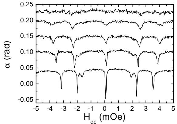
FIG. 2: The phase angle  $\alpha$  as a function of the external magnetic field applied parallel to  $c$ -axes of  $65\mu\text{m}$ -wide bridge across an asymmetric  $45^\circ$   $\text{YBa}_2\text{Cu}_3\text{O}_x$  grain boundary. From top to bottom the data correspond to  $T=40, 30, 20, 10,$  and  $4.2$  K. The data are vertically shifted for clarity.
