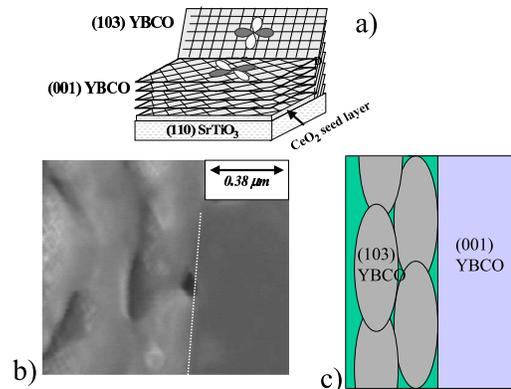
FIG. 1: a) Sketch of the investigated bi-epitaxial grain boundary where a  $45^\circ$  *c*-axis tilt accompanies the  $45^\circ$  *a*-axis tilt; in b) a Scanning Electron Microscope image relative to the this GB is shown. The elongated grains on the left typical of the (103) growth may generate clean interfaces with reduced faceting, as evident also by the sketch in c).
