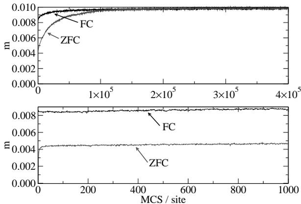
FIG. 13: Long-time (upper panel) and short-time (lower panel) behavior of the magnetization per spin versus time at  $T/J' = 10^{-6}$  for a FC and a ZFC protocol. The external field has magnitude  $h/J' = 10^{-2}$ .
