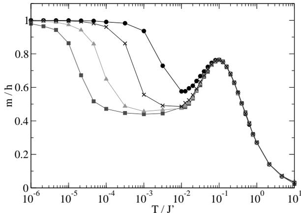
FIG. 9: The equilibrium magnetization per spin in units of  $h$  as a function of the temperature, for  $h/J' = 10^{-2}$  (squares),  $2 \times 10^{-2}$  (triangles),  $5 \times 10^{-2}$  (crosses),  $10^{-1}$  (circles). Lines are guides to the eye.
