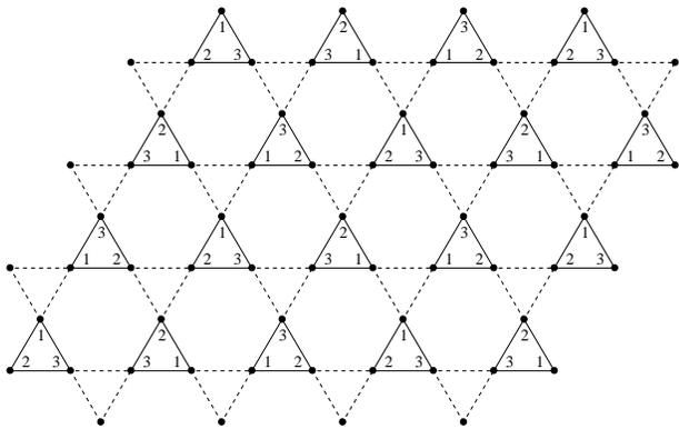
FIG. 1: The *trimerized kagome* lattice. The solid and dashed lines indicate the antiferromagnetic coupling  $J$  and  $J'$ , respectively. The numbers 1, 2 and 3 indicate the site indexing inside the elementary triangles which defines the gauge (see section II).
