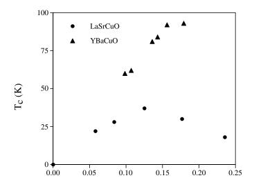
Fig. 1: Phase diagram for  $La_{2-x}Sr_xCuO_4$  and  $YBa_2Cu_3O_{6+y}$  as derived from NMR data shown in Tab. 1. The transition temperature  $T_c$  is plotted against the hole content per CuO<sub>2</sub>, given by  $\delta$  as determined from NMR data.
