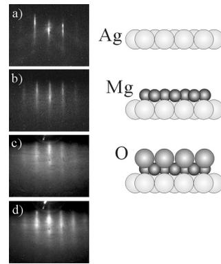
FIG. 4. A typical sequence of RHEED patterns and schematic models during the growth of the MgO film on Ag(111) at a substrate temperature of 300 K. a) Ag(111), b) 1 ML MgO/Ag(111), c) 2 ML MgO/Ag(111), d) 10 ML MgO/Ag(111). The incident beam was parallel to the [110] azimuth of the Ag(111).
