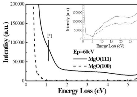
FIG. 6. EEL spectra of the polar MgO (111) surface (line). The primary electron energy was 60 eV. Spectra of MgO (100) surface is shown for comparison (dot line).
