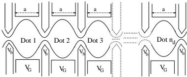
FIG. 1. Schematic diagram of a multiple dot system ( $n_d$  dots) defined on a two dimensional electron gas. The barriers forming the dots are denoted as  $V_b$  and the gate voltages controlling the density in the dots are denoted as  $V_G$ .
