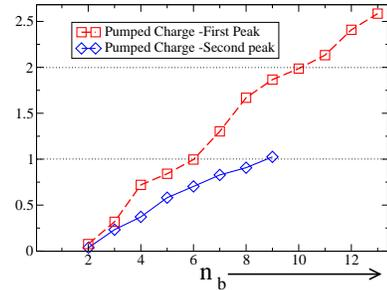
FIG. 3.  $Q$  (in units of  $e$ ) as a function of the number of barriers  $n_b$ . The top line is for the first peak and the line below is for the second peak. The parameter specifications are the same as for Fig.2.
