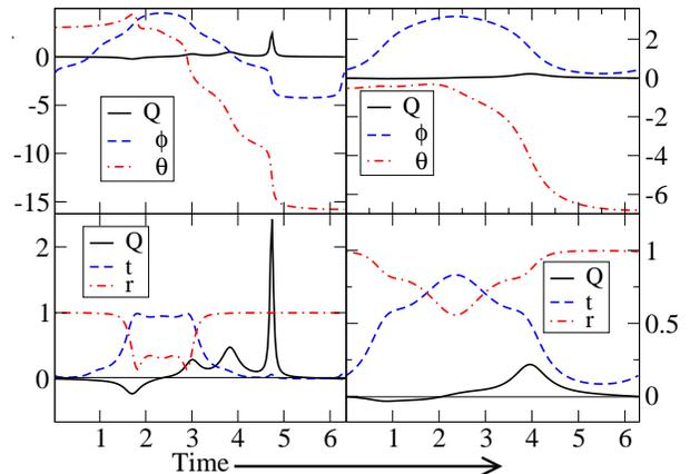
FIG. 4. Transmission and reflection amplitudes ( $t$  and  $r$ ) and phases ( $\phi$  and  $\theta$ ) and the pumped charge  $Q$  as a function of time (for a single period  $\tau = 2\pi$ ) for  $n_b = 10$  barriers (left panel) and  $n_b = 4$  barriers (right panel).  $Q$  is measured in units of  $e$  and  $\phi$  and  $\theta$  in radians.
