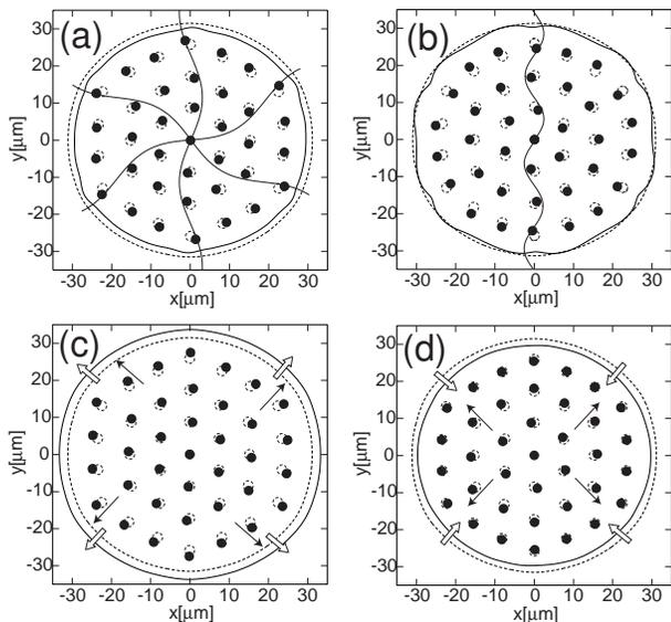
FIG. 2: Oscillation patterns for the (a) lowest TK, (b) second TK, (c) lowest BR, and (d) second BR modes are indicated by the filled circles and solid lines. Empty circles and dotted lines correspond to the equilibrium state,  $\phi_g$ .
