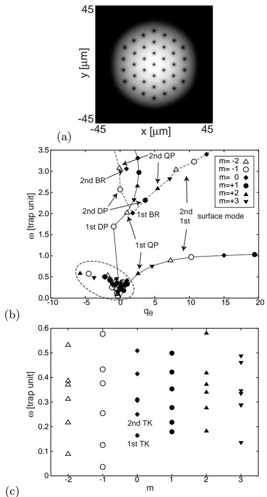
FIG. 1: (a) Density profile of the condensate with 37 vortices at  $\Omega = 0.7\omega_r$ . (b) Collective excitations up to  $\omega = 3.5\omega_r$ . (c) Lowest excitations marked by a dotted line as functions of  $q_\theta$  are displayed as functions of the symmetry index  $m$ . Here, TK, BR, DP, and QP denote the Tkachenko, breathing, dipole, and quadrupole modes, respectively.
