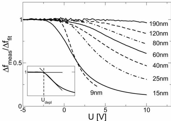
FIG. 2: Relative Kelvin probe. The data from Fig. 1 are divided by their respective parabolic fit. *Inset*: The position where the depletion sets in,  $U_{\text{depl}}$ , is defined as indicated as the point where the tangent to the curve crosses the  $y = 1$  axis.
