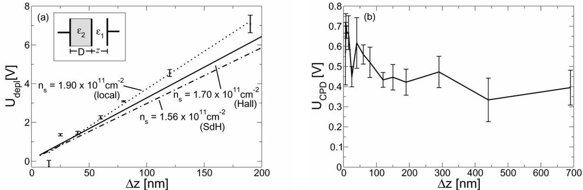
FIG. 3: *a)* Depletion voltage plotted versus the tip-sample distance at which the Kelvin probe was recorded. The electron density extracted from the transport data is  $n_{\text{Hall}} = 1.70 \cdot 10^{11} \text{ cm}^{-2}$  and  $n_{\text{SdH}} = 1.56 \cdot 10^{11} \text{ cm}^{-2}$ . This leads to the solid lines in the graph. Inset: Model geometry. *b)* Contact potential difference  $U_{\text{CPD}}$  plotted as a function of  $\Delta z$ .
