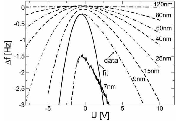
FIG. 1: Kelvin probe at different tip-sample distances. On the vertical axis the frequency shift  $\Delta f$  is plotted versus the bias voltage  $U$  on the horizontal axis. The solid line indicates the parabolic fit to the data taken at 9 nm tip-sample separation. We choose the sign of the voltage always with respect to the 2DEG, i.e., a negative voltage indicates that the negative contact is connected to the electron gas.
