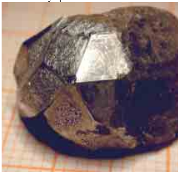
Fig. 1 si -Ho-Mg-Zn: Centimeter sized single crystal of triacontahedral morphology
