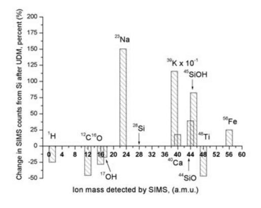
Fig. 2. Effect of UDM on SIMS spectrum from Cz-Si (sample Cz-p-Si-2K). Negative values mean that the counts became lower after UDM, positive values – counts became higher after UDM.
