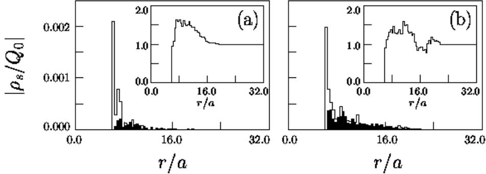
**Figure 3.** The distribution functions of the counterions (open bars) and coions (shaded bars) for the rod macroion with double helix charges whose surface charge is equal to that of the DNA. These correspond to the filled circles in Fig.2 with the ionic strength (a)  $n_{zI} \sim 0.005a^{-3}$  and (b)  $n_{zI} \sim 0.013a^{-3}$ .
