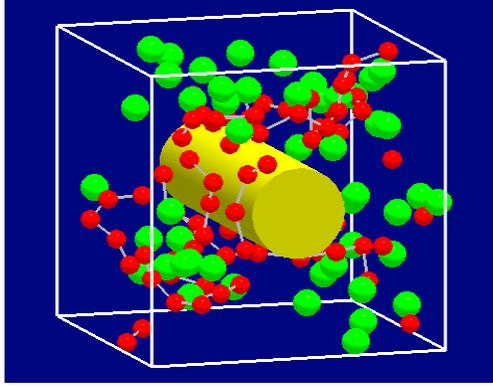
**Figure 5.** A cylindrical macroion with long polyelectrolyte cations of unit charges (red) and isolated anions (green) has reversed mobility. The surface charge density of the macroion with double helix charges,  $\sigma_{rod} \sim 0.02e/a^2$ , is approximately that of the DNA. The long chains of polyelectrolyte mechanically wind around the rod. The radius and number of anions are  $a^- = 1.5a$  and  $N^- = 60$ , respectively [neutral particles are not shown].
