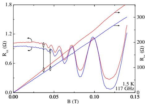
FIG. 4: The periodicity of radiation induced  $R_{xx}$  oscillations appears insensitive to the electron density,  $n$ . Here, increasing the slope of  $R_{xy}$  vs.  $B$  corresponds to decreasing  $n$ .
