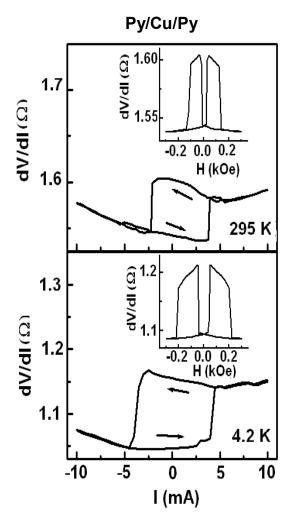
Fig. 1. Py/Cu/Py data at 295K and 4.2K showing normal switching for dV/dI vs I at H = 50 Oe (main figures) and also for dV/dI vs H at I = 0 (insets). (From Urazhdin et al.<sup>24</sup>).
