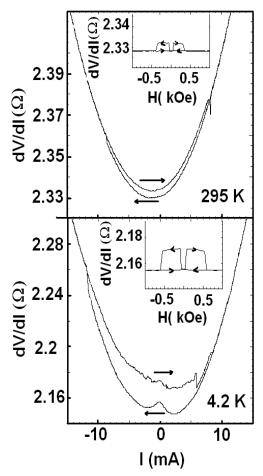
Fig. 2. Fe(Cr)/Cr/Fe(Cr) data at 295K and 4.2K showing inverted switching for dV/dI vs I at H = 0 (main figures) but normal dV/dI vs H at I = 0 (insets).
