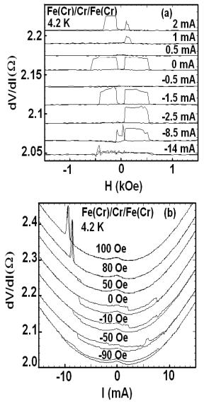
Fig. 3. Fe(Cr)/Cr/Fe(Cr) data at 4.2K showing: (a) normal MR for dV/dI vs H at various I, but (b) inverted switching for dV/dI vs I at various H. Curves in (a) for  $I \neq 0$  and in (b) for  $H \neq 0$  are shifted vertically for clarity.
