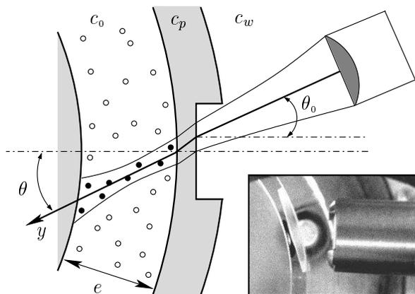
FIG. 4: Experimental setup for USV in complex fluids sheared in the Couette geometry.  $c_0$ ,  $c_p$ , and  $c_w$  stand for the speed of sound in the complex fluid, in Plexiglas, and in water respectively. The inset shows a picture of the transducer and the stator as seen from above once the rotor has been removed.
