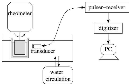
FIG. 3: Electronic system used for high-frequency USV.
