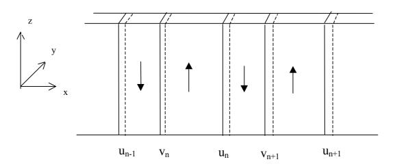
Fig. 1. The domain structure. The domain wall displacements are shown by dashed lines. The arrows show the magnetization directions in domains.
