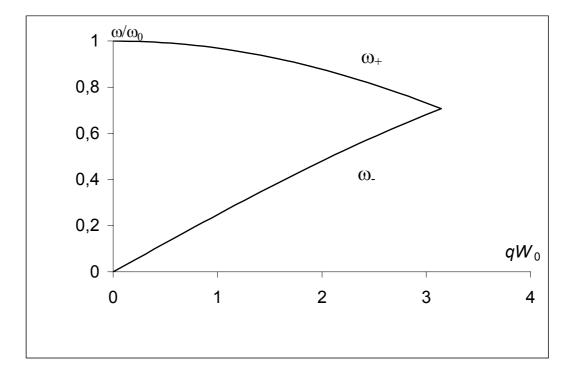
Fig. 2. Domain wall oscillation spectra.
