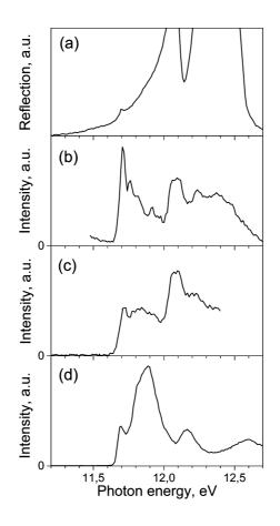
Figure 1: (a) – Reflection of solid Ar. (b) – Excitation spectrum of *W*-band. (c) – Spectrum of photon yield measured at hv=11.47 eV. (d) – Excitation spectrum of *M*-band. All data were measured at T=10 K.
