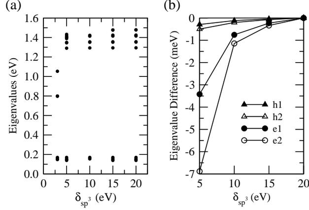
FIG . 7: (a) Electron energy versus dangling-bond energy shift  $\delta_{sp^3}$ , (b) Variations of the ground and excited electron (e1, e2) and hole (h1, h2) energies with respect to energy shift. A energy shift larger than 5 eV eliminates surface states in the middle of the gap between 0.2 and 1.2 eV. The electron and hole energies vary only by a few meV when the energy shift varies from 5 to 20 eV.
