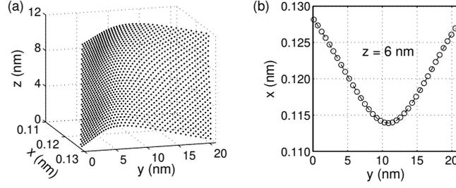
FIG. 6: Atomic positions at the boundary plane of the truncated GaAs buffer: (a) 3-D visualization of the boundary plane, (b) a slice through a plane with  $z$  about 6 nm. The plane is bent due to non-uniform strain generated by the lattice mismatch between the InAs dot and GaAs buffer. The variation of the atomic positions along the  $x$  axis is about 5% of the unstrained bond length of 0.24 nm.
