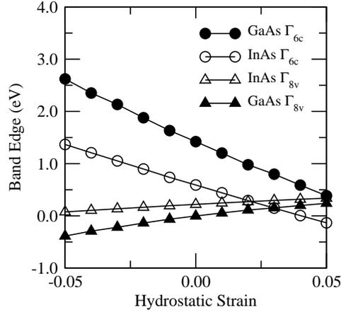
FIG . 3: Conduction and valence band edges at  $\Gamma$  with respect to hydrostatic strain for bulk InAs and GaAs. The compressive strain increases the direct band gap while the tensile strain decreases the gap.
