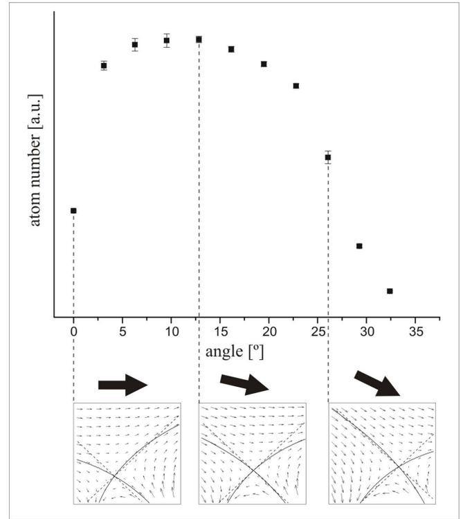
FIG. 3: Top: The number of atoms is plotted versus the tilting angle between the bias field and the plane of the U-shaped wire. For these measurements the U-current was 55A, the bias field strength 13G. Bottom: Corresponding vector field plots for three different angles (0, 13, 26) as indicated by the arrows. The maximum number of atoms is trapped at a bias field angle of 13 where the shape of the field is closest to an ideal quadrupole field.
