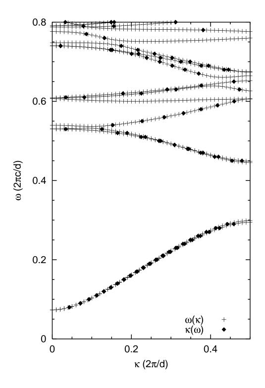
Figure 1: Band structure of an intersecting square-rod model calculated as ! (k) and k(!) for realk = (0:1;0; )2 =d. The number of the reciprocal lattice points is 9 9, and other parameters are the same as in ref.[5].
