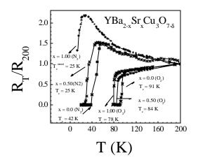
Fig. 2 Resistance versus temperature plots for both  $O_2$  and  $N_2$  annealed  $YBa_{2-x}Sr_xCu_3O_{7-\delta}$  samples
