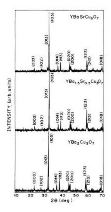
Fig.1 X-ray diffraction patterns for Q-annealed YBa<sub>2-x</sub>Sr<sub>x</sub>Cu<sub>3</sub>O<sub>7-δ</sub> samples
