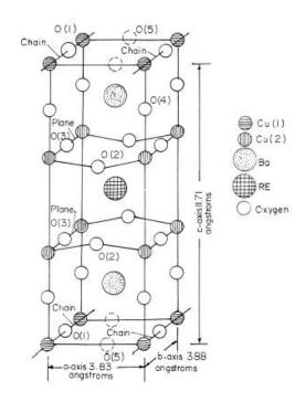
Fig.1 Schematic unit cell of REBa<sub>2</sub>Cu<sub>3</sub>O<sub>7</sub>.
