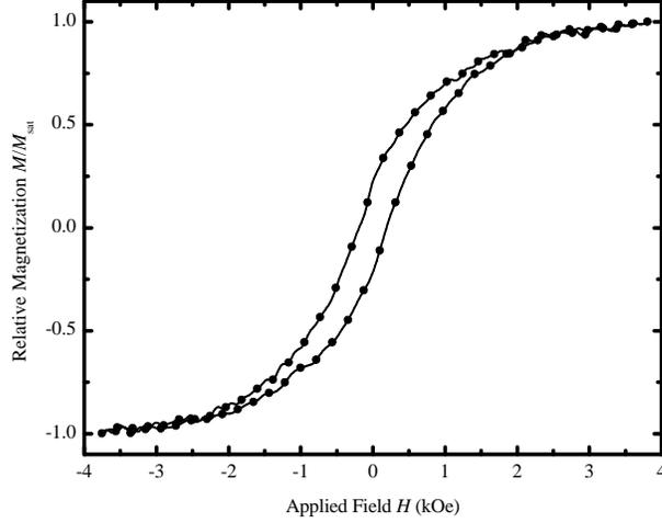
Fig. 1. Hysteresis loop of  $a\text{-Co}_{25}\text{Nb}_{75}$ .
