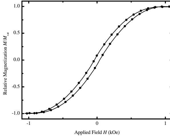
Fig. 3. Hysteresis loop of  $a\text{-Co}_{80}\text{Nb}_{20}$ .
