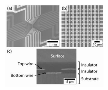
FIG. 1. (a) Micrograph of a  $10 \times 10$  microelectromagnet matrix with its leads. (b) A closeup of the matrix: two layers, each with 10 Au wires, are aligned perpendicular to each other, separated and topped by insulating layers. The width and the pitch of the wires are 5 µm and 10 µm, respectively. (c) Cross section of the matrix along a diagonal direction; the top and bottom wires are indicated along with the substrate, two insulating layers, and the top surface.
