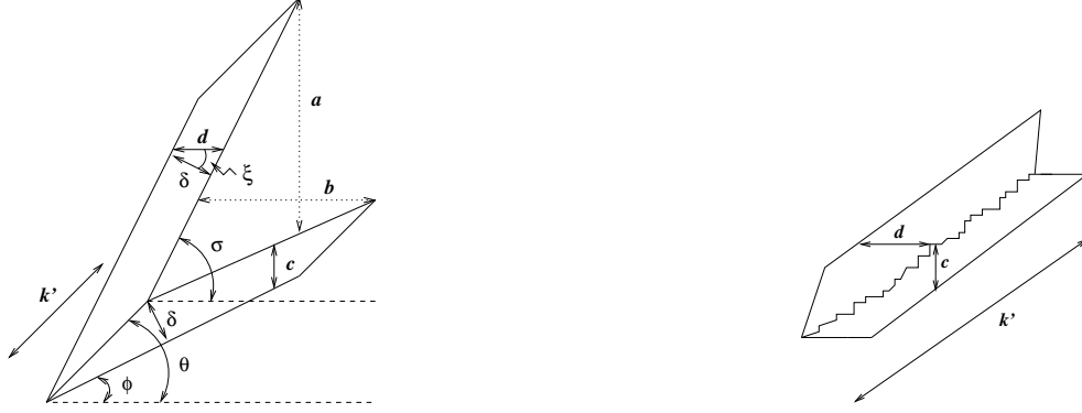
FIG. 10: Typical jam configurations. For type I jams, shown in (a), c = d = k^0 . For type II jams, shown in (b), d = d_{\max} and c = c_{\max} . Knowing the slopes of the lines in (a), s = 1 , s_r = 2 , and s_b = 1/2 , we can determine all of the angles: \delta = \tan^{-1}(1/2) , \xi = 4 , \sigma = \tan^{-1} 2 , and \theta = (\pi/2 - \tan^{-1} 2) .
