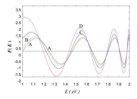
FIG 2: Bound state energies of a 20 atom dot attached to two leads of same onsite
