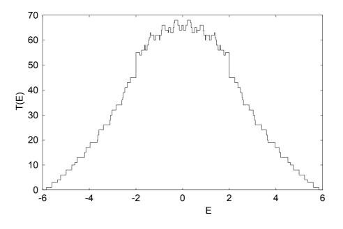
FIG 4 : this figure shows the transmission coefficient T(E) vs. E(eV)[Fermi energy] for the following specific parameters (ideal wire):
