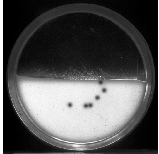
FIG. 1: Ring of segregation of 1.5-mm large tracer beads (Glass) in a bed of 90- \mu m small Glass beads, in a quasi2D (2 dimensions) drum. The radial location of tracers is precisely defined (note that the upper bead is still in the flowing layer). The position is very sensitive to the value of the size ratio [6] and of the density ratio [this paper]. The variation of the ring radius is a powerful means to study the geometrical effect of segregation by making an equivalence with the variation of position induced by a change of density.
