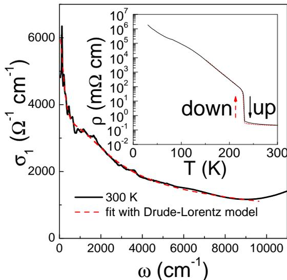
FIG. 1: (Color online) The optical conductivity spectrum of  $\text{CuIr}_2\text{S}_4$  at 300 K. Dashed curve is a fit to the data using two Drudes and one Lorentz components. The inset shows T-dependence of dc resistivity as the sample was cooled down and warmed up.
