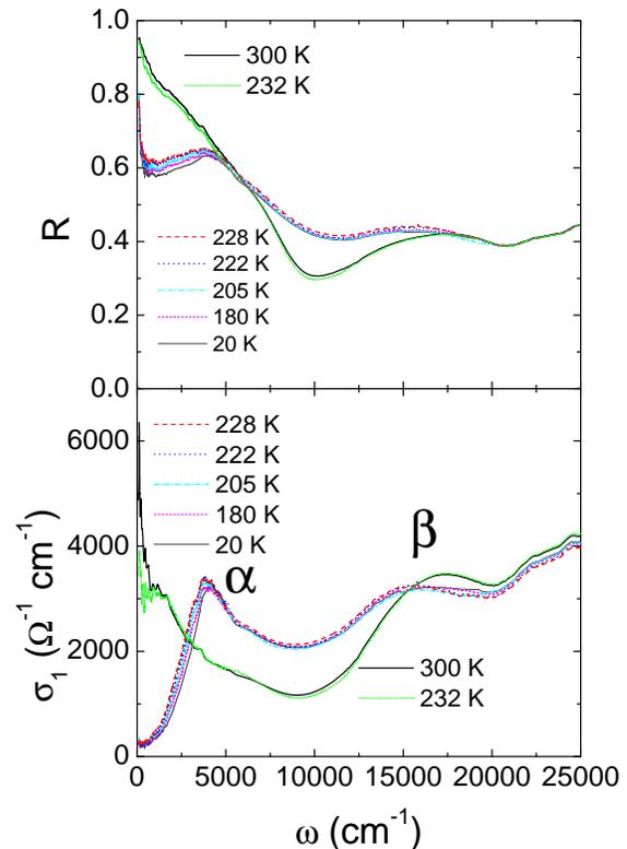
FIG. 2: (Color online) Temperature dependence of the reflectivity spectra (up panel) and optical conductivity spectra (bottom panel) for a  $\text{CuIr}_2\text{S}_4$  single crystal with  $T_{MI}=230 \text{ K}$ . Abrupt spectral change occurs at  $T_{MI}$ .
