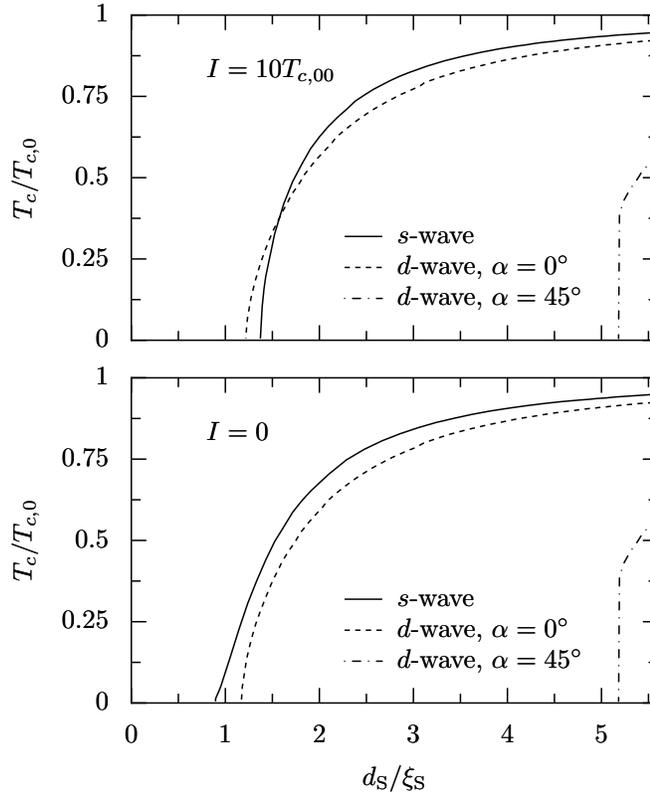
**Figure 3.** The critical temperature of a thin superconducting layer on top of a bulk ferromagnet ( $I = 10T_{c,0}$ ,  $d_F \rightarrow \infty$ ) as a function of the layer thickness,  $d_S$ , which is normalised by the superconducting coherence length  $\xi_S$  (upper panel). For comparison the critical temperature is also shown for  $I = 0$  (lower panel).
