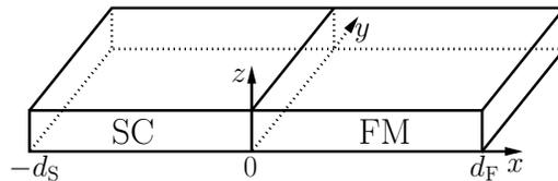
**Figure 1.** A bi-layer consisting of a superconductor of thickness  $d_S$  and a ferromagnetic metal of thickness  $d_F$ . The interface between both materials (at  $x = 0$ ) is assumed to be completely transparent, and the sample is translationally invariant in  $y$ - and  $z$ -direction.
