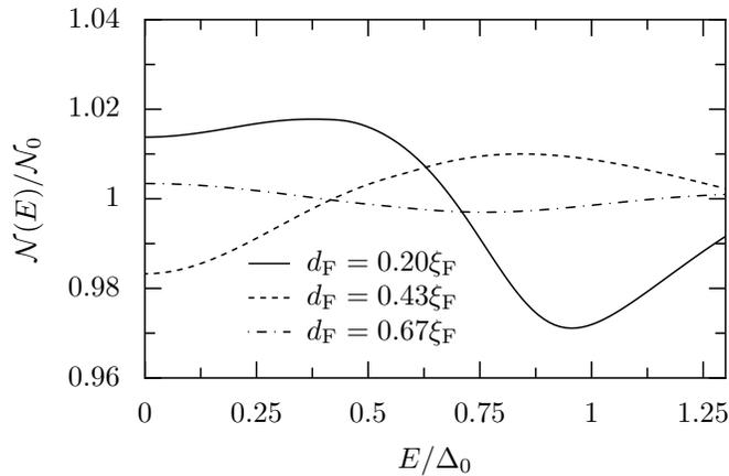
**Figure 6.** The density of states at  $x = d_F$  for an unrotated  $d$ -wave symmetry of the order parameter. These values of  $d_F$  correspond to the first two minima ( $d_F = 0.20, 0.67\xi_F$ ) and the first maximum ( $d_F = 0.43\xi_F$ ) of the critical temperature.
