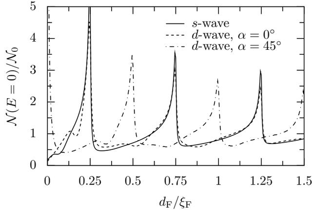
**Figure 2.** The density of states at  $E = 0$  is shown as a function of the ferromagnetic layer thickness with  $\xi_F = \pi v_F/I$ . The  $s$ -wave and the unrotated  $d$ -wave case are almost identical with maxima at  $d_F = (1/2 + k)\xi_F/2$ , where  $k$  is an integer; for a rotated  $d$ -wave order parameter the maxima are shifted to  $d_F = k\xi_F/2$ . For the plot we added a finite imaginary part to the energy ( $E \rightarrow E + i0.01T_c$ ).
