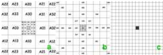
FIG. 3: Linear decomposition hierarchies with 4-fold symmetry: (a) 4 \times 4 , (b) 8 \times 8 , (c) 16 \times 16 .
