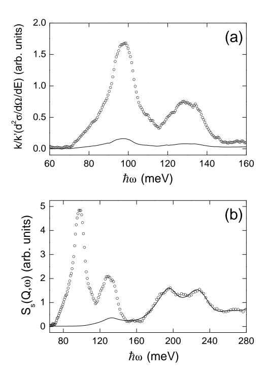
FIG.1: Neutron scattering spectra from LiH at T = 20:1(1) K: (a) TO SCA-II experimental data (circles) together with the estimate of the multiple scattering contribution (line); (b) experimental scattering law (circles) and its multiphonon component (line).
