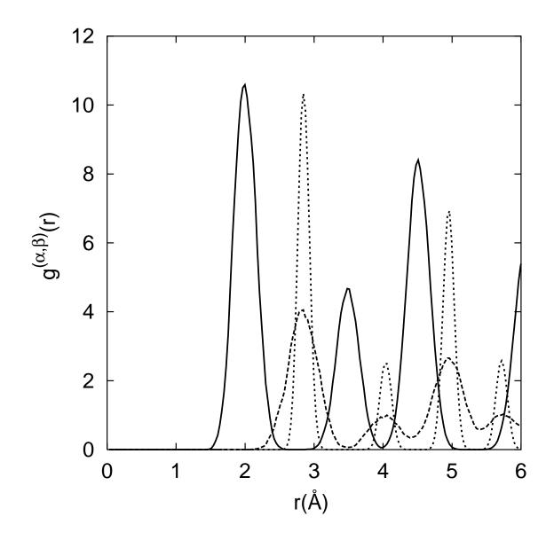
FIG. 3: Two-body radial distribution functions in LiH:  $g^{(H;Li)}(r)$ , solid line;  $g^{(H;H)}(r)$ , dashed line;  $g^{(Li;Li)}(r)$ , dotted line.
