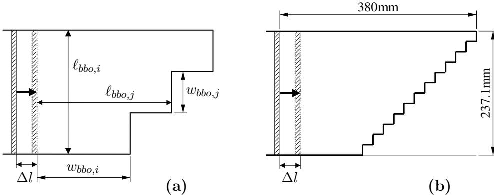
Fig. 1. Investigated billiards with genus  $g = 3$  and  $g = 12$ . One wall was shifted in steps of 0.25 mm. Some of the widths  $w_{bbo}$  and the length  $l_{bbo}$  of the main bouncing ball orbits, taken into account for the unfolding of the spectra, are shown.
