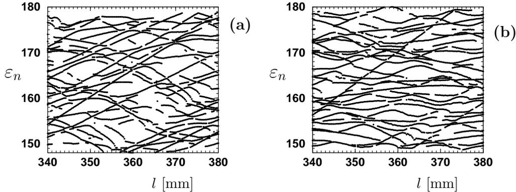
Fig. 2. The unfolded energy levels  $\varepsilon_i$ ,  $i = 151, \dots, 180$  as a function of the billiard length  $l$  for the  $g = 3$ -system (a) and the  $g = 12$ -system (b). It can be recognized that there are more straight lines in the spectrum of the billiard with  $g = 3$ .
