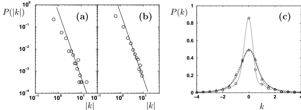
Fig. 4. Distribution of the absolute value of the scaled curvatures  $|k|$  in a double logarithmic scale for the  $g = 3$  -billiard (a) and the  $g = 12$  -billiard (b). The solid line indicates a  $|k|^{-3}$  behavior as expected for GOE systems. Case (c) shows the distribution of  $k$  for  $g = 3$  (circles) and  $g = 12$  (triangles) for  $\varepsilon \in [350, 400]$ . The solid line shows the theoretical prediction for a GOE system (see Eq. (2)).
