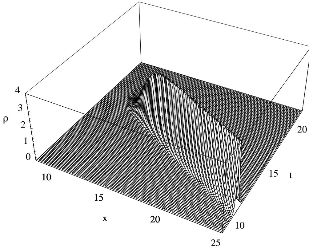
Figure 2: The soliton propagates to the left until it reaches the PML at  $x = 10$ . Here it becomes 'stuck' and  $\rho$  drops sharply, to about 0.03% of the original value.
