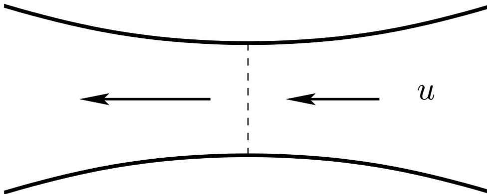
Figure 1: Schematic illustration of a supersonic nozzle. The flow velocity  $u$  exceeds the speed of sound at the throat of the nozzle
