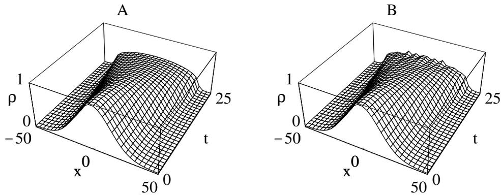
Figure 3: These pictures show the expansion of a condensate in a domain 100 space units wide. In (A) the PML is placed in a 5-unit-wide region on the left- and right-hand sides of the domain, while in (B) the PML is not present, which causes monotonically growing instabilities to be seen as time proceeds. The expansion with the PML is practically identical to the expansion in a 1000-unit-wide domain, where the condensate does not touch the sides of the computational domain.
