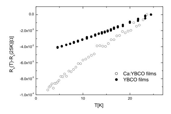
Fig. 3. The change of the surface resistance for two types of samples: open circles for overdoped Ca-YBCO films, filled circles for optimally doped YBCO films.
