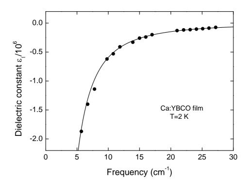
Fig. 1. The real part of the dielectric function versus frequency for a thin Ca overdoped YBCO film, T= 2 K. Dots show experiment, lines show the fit to expression  $\varepsilon_1 = -\omega_p^2 / \omega^2$  describing the response of superconducting condensate [16], as discussed in the text. The best fit yields  $\lambda(0) = 2070 \text{ Å}$ .
