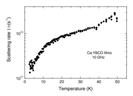
Fig. 4. Temperature dependence of the scattering rate of uncondensed carriers for the films which are almost free of a-axis grains. The data were taken at *10 GHz*.
