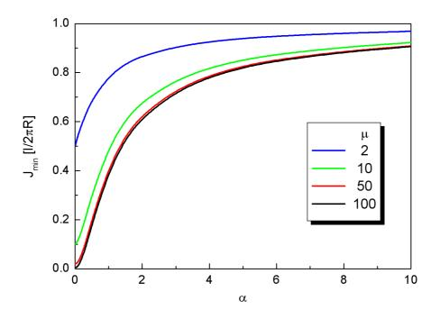
Fig. 4. Minimum value of the sheet current of the superconducting filament,  $J_{min}$ , as a function of the distance between the filament and the magnet relative to the radius of the filament,  $\alpha$ , for different values of the relative permeability,  $\mu$ , specified in the legend. The minimum value of the sheet current in the absence of the magnet (i.e. for  $\mu = 1$ ), adopted independently of  $\alpha$ , is unity.
