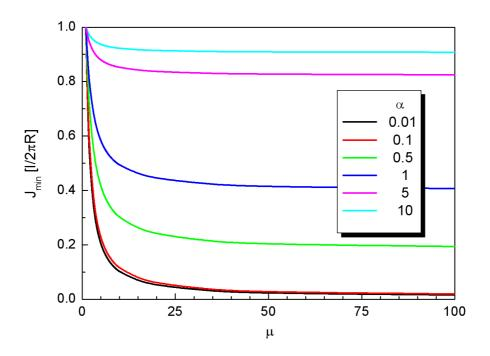
Fig. 5. Minimum value of the sheet current of the superconducting filament,  $J_{min}$ , as a function of the relative permeability,  $\mu$ , for different values of the distance between the filament and the magnet relative to the radius of the filament,  $\alpha$ , specified in the legend. The minimum value of the sheet current in the absence of the magnet (i.e. for  $\mu = 1$ ), adopted independently of  $\alpha$ , is unity.
