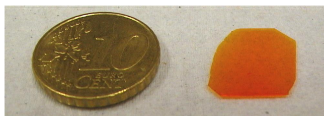
FIG. 5: A \text{cm}^2 -sized platelet-shaped tetracene single-crystal grown by physical vapor transport.
