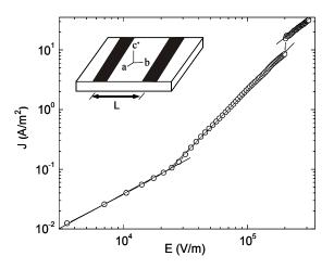
Fig 2. Current density vs. electric field for pentacene single crystal at room temperature. The solid lines represent the fits for the three different regimes. The inset shows experimental configuration of the a, b, and c\*-axis, and the contacts. The hole-injecting electrodes are 40-50 nm thick gold.
