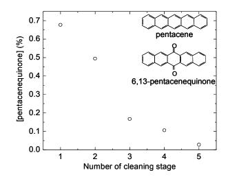
Fig1. 6,13-pentacenequinone concentration in pentacene in different stages of purification: 1-as received, 2-single sublimation clean, 3-double sublimation clean, 4-crystal grown from untreated powder, 5-crystal grown from doubly cleaned powder. The inset represents the Lewis structure of pentacene and 6,13-pentacenequinone.
