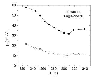
Fig 3. Temperature dependence of the electrical hole mobility for pentacene single crystal using the actual crystal thickness ( $\circ$  open circles) and effective thickness ( $\bullet$  closed circles).
