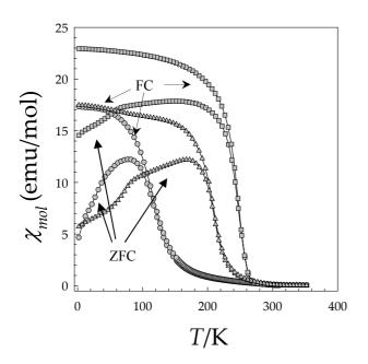
Fig. 1 ZFC and FC curves for oxygen annealed  $La_{1-x}Na_xMn_{1-y}Ru_yO_{3+\delta}$  samples with x = 0.05 and y = 0 (circles), 0.05 (squares) and 0.15 (triangles).
