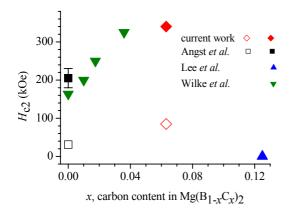
FIG. 5. Upper critical field  $H_{c2}$  of Mg(B<sub>1-x</sub>C<sub>x</sub>)<sub>2</sub> as a function of carbon content. Open symbols correspond to  $H_{c2}^{\parallel c}(0)$  (squares – Ref. 4). Full symbols correspond to  $H_{c2}^{\parallel ab}(0)$ (squares – Ref. 27, triangles up – Ref. 15, triangles down – Ref. 16).
