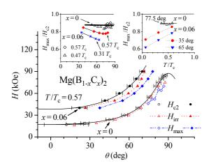
Fig. 3. Angle dependence of upper critical field  $H_{c2}$  (circles), the irreversibility field  $H_{irr}$  (triangles), and the peak maximum field  $H_{max}$  (diamonds) at  $0.57T_c$  for Mg(B<sub>0.94</sub>C<sub>0.06</sub>)<sub>2</sub> (full symbols) and for MgB<sub>2</sub> (open symbols). Full lines are fits of the theoretical  $H_{c2}(\theta)$  dependence [Eq. (1)] Dashed lines are guides for eye. Left inset:  $\theta$  dependence of the
