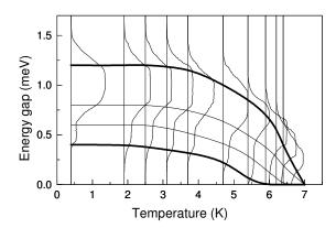
Fig. 5. Evolution with temperature of NbSe<sub>2</sub> gap distributions. Lines indicating the evolution of the main features are sketched.
