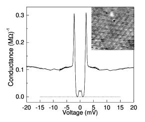
Fig. 3. Pb-NbSe<sub>2</sub> conductance curve in tunneling regime at 4.2 K. Inset:  $10 \times 10 \text{ nm}^2$  STM topographic image of a NbSe<sub>2</sub> surface using a Pb tip.
