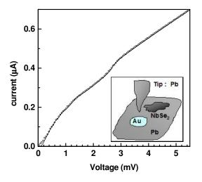
Fig. 1. I-V curve corresponding to a single atom contact (circles), and the fitting using three quantum channels with transparencies 0.87, 0.26 and 0.05 (solid line). Inset: configuration of the composite sample.
