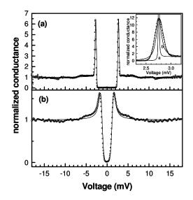
Fig. 2. Pb-Pb (a) and Pb-Au (b) conductance curves in tunneling regime at 2K (dots: experiment; line: fit). Inset: detail of the gap edge fitted using a gaussian distribution, and BCS curves obtained using a single value of  $\Delta$  (1.375 meV) and a lifetime parameter,  $\Gamma$ . Curve (a),  $\Gamma$ =1 $\mu$ V; curve (b),  $\Gamma$ =30 $\mu$ V.
