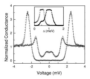
Fig. 4. Pb-NbSe<sub>2</sub> conductance curves at 1.9K and 6K (experiment :dots; fitting: line). Inset: gap distributions obtained in the fitting procedure (solid, 1.9K; open, 6K).
