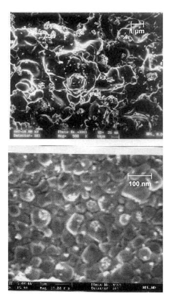
Fig. 2 : SEM micrographs of (a) SRA and (b) SRAC phosphors.
