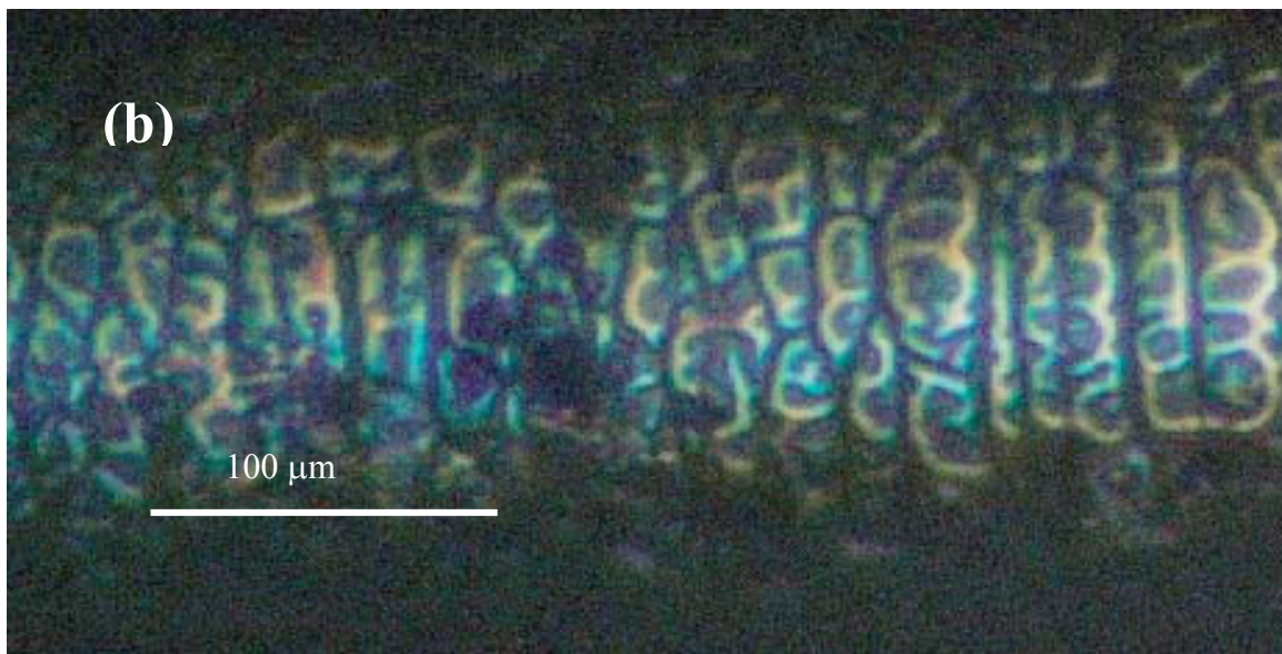
Fig. 7: An optical microscopy image of the boron wire (a) and of a MgB 2 wire segment coated with an evaporated ~120 nm gold layer (b).
