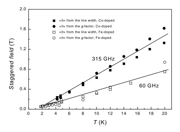
Fig. 2. Temperature dependence of the staggered field in CuGeO<sub>3</sub>:Co and CuGeO<sub>3</sub>:Fe from EPR measurements. Solid lines are guides for the eyes.
