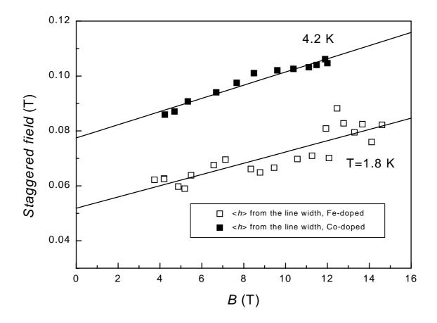
Fig. 3. Field dependences of the staggered field in doped CuGeO<sub>3</sub>. Solid lines represent best fits with equation (5).
