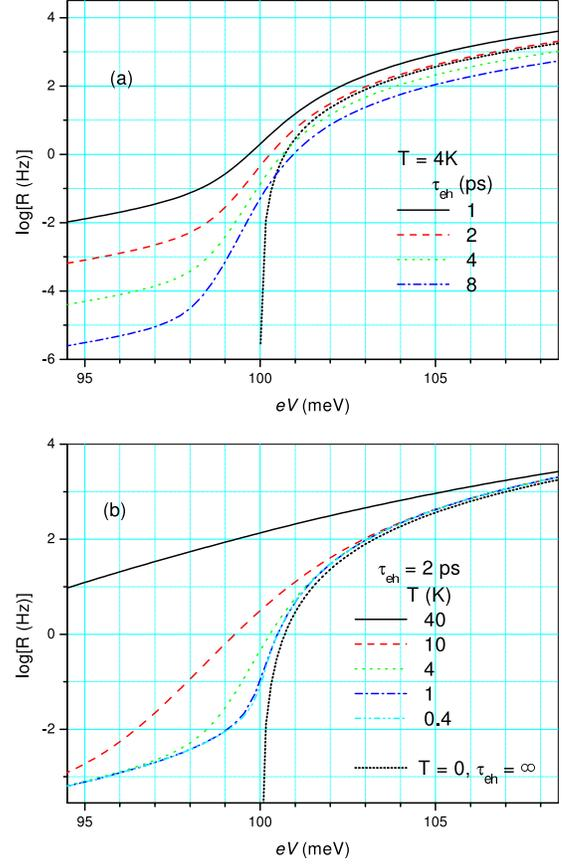
FIG. 4: Voltage dependences of the logarithm of the transfer rate, calculated for bath temperature  $T = 4$  K and different vibrational lifetimes (a); for  $\tau_{eh} = 2$  ps and different temperatures (b). Short dotted line in both panels shows the transfer rate in the simple approximation neglecting the phonon broadening effect,  $\tau_{eh} = 1$ , and at  $T = 0$ ,  $R(V) / (j_e V)^n$ ,  $n = 3$ .
