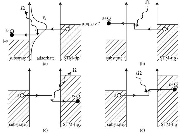
FIG. 1: Schematic representation of the inelastic electron transfers through the adsorbate from tip to substrate with emission and absorption of phonons  $R_{ts}^+$  and  $R_{ts}^-$ , (a) and (b), respectively. Same from substrate to tip with emission and absorption of phonons  $R_{st}^+$  and  $R_{st}^-$ , (c) and (d), respectively.
