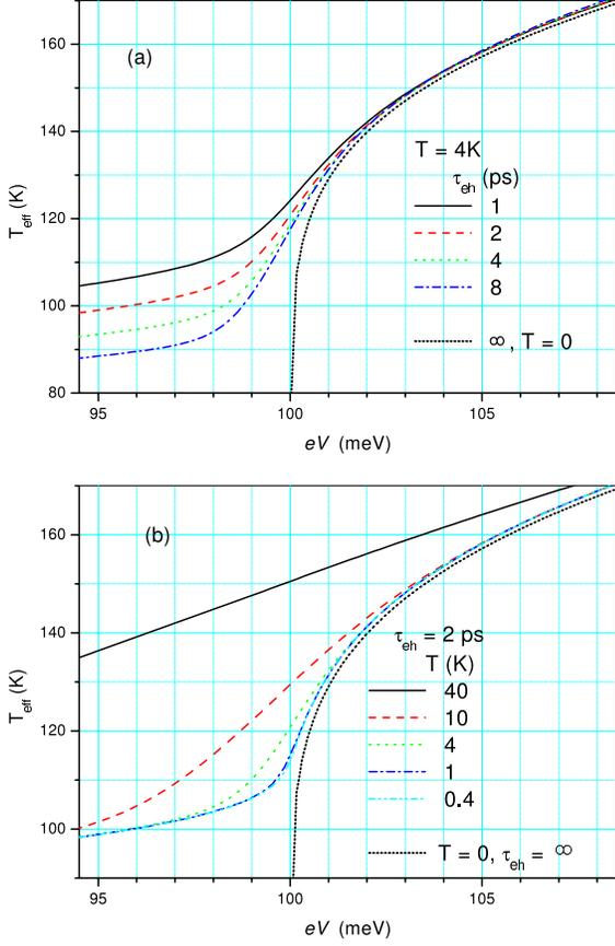
FIG. 3: Voltage dependences of the effective temperature, calculated for bath temperature  $T = 4$  K and different vibrational lifetimes (a); for  $\tau_{eh} = 2$  ps and different temperatures (b). Short dotted line in both panels shows the effective temperature in the simple approximation neglecting the phonon broadening effect,  $\tau_{eh} = 1$ , and at  $T = 0$ ,  $i_{iet}(V) / (j_e V)^3$ .
