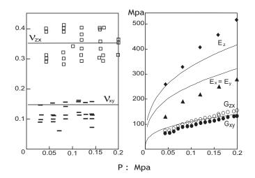
FIG. 1: The Poisson ratios  $_{zx}$ ;  $_{xy}$ , the Young moduli  $_{zz}$ ;  $_{Ex}$  =  $_{Ey}$ , and the shear moduli  $_{zx}$ ;  $_{Gxy}$ , measured [8] with Ham River sand at  $_{xx}$  =  $_{zz}$  = 0.45 and a void ratio of 0.66, compared to the calculated curves assuming  $_{Ex}$  =  $_{Ex}$  = 6800M pa, with  $_{Ex}$  =  $_{Ex}$  =
